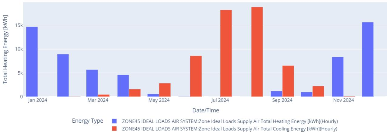
Figure 48: Monthly THE and TCE for the classroom used for calibration, Building O9.
