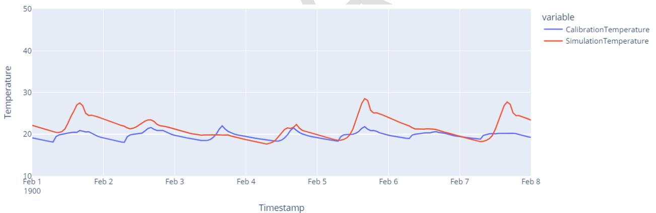
Figure 20: Hourly Real vs Simulated data before the model calibration (winter week), Building 09.
