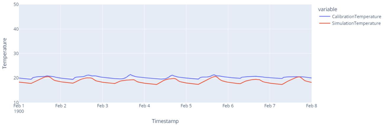
Figure 25: Hourly Real vs Simulated data after the model calibration (winter week), Building 10.
