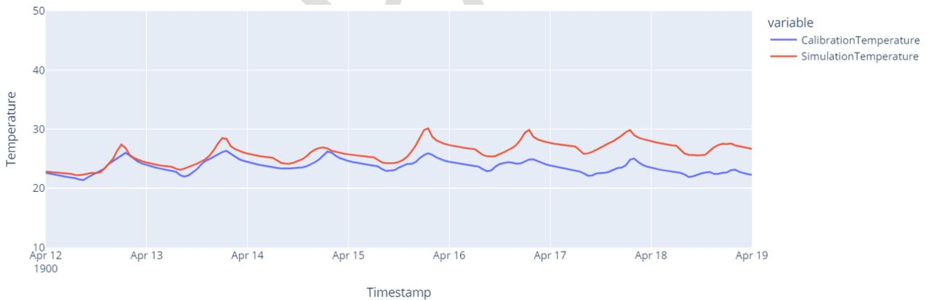
Figure 18: Hourly Real vs Simulated data before the model calibration (spring week), Building 10.
