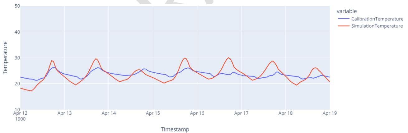
Figure 32: Hourly Real vs Simulated data after the model calibration (spring week), Building 09.
