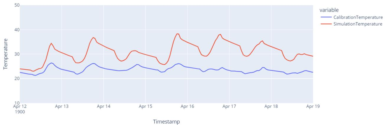
Figure 22: Hourly Real vs Simulated data before the model calibration (spring week), Building 09.
